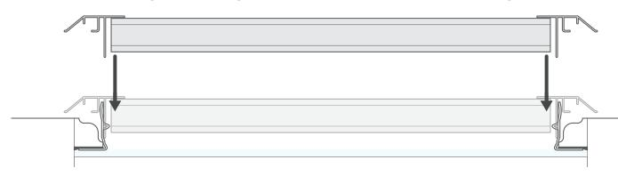
Push the frame towards the window until the oval slots lock onto the prongs of each of the brackets. The installation of the blind is now complete.
