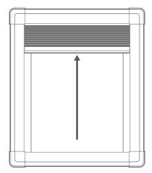
Stand the assembled frame upright and raise it fully to the top. If the blind starts to lower slightly of its own accord, the tension will need a small adjustment.
